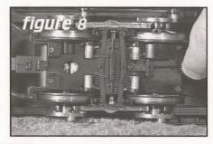
Now, using light gear oil, lubricate the crankpins that connect the side rods to the wheels (figure 11).
