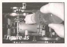
Next, take heavy gear oil and put a drop on all of the visible gears (figure 15).
