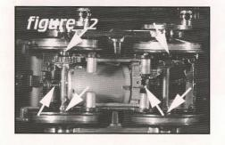
Continuing with the light gear oil, lubricate all of the mating and telescoping surfaces along the center drive shaft. Again, a single drop or two at each joint will suffice. And don't forget the valve gear at the bottom of the V 2 cylinders (figures 13 & 14). Be sure to lubricate all of the bearing surfaces.
